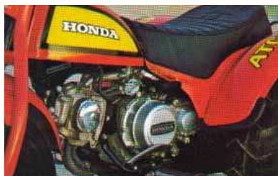
Rugged 89 cc overhead cam four-stroke with dual range transmission. ATC 90 K1
